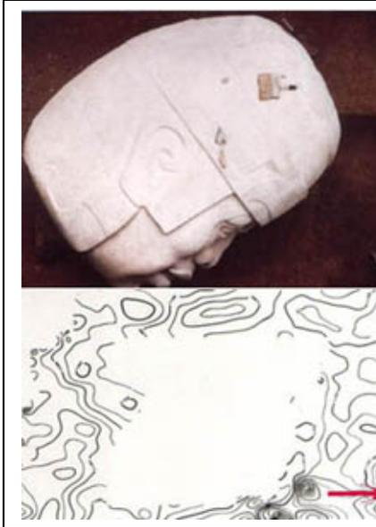
**The best preserved Olmec head found weighed 10 tons and was buried 16 feet deep at the anomaly indicated on the magnetic intensity contour map. (The blank area was covered by a pond where no measurements were taken.) Graphic proof of Breiner's law of search: the find is always at the edge of the survey area.**
